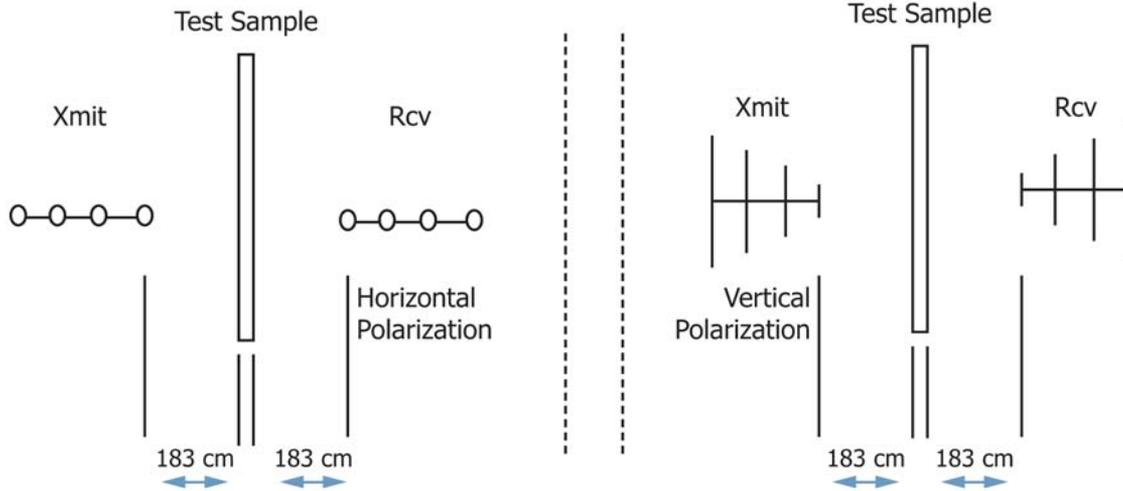
FIG. 5 Plane Wave Antenna Polarizations (Log Periodic et al)
