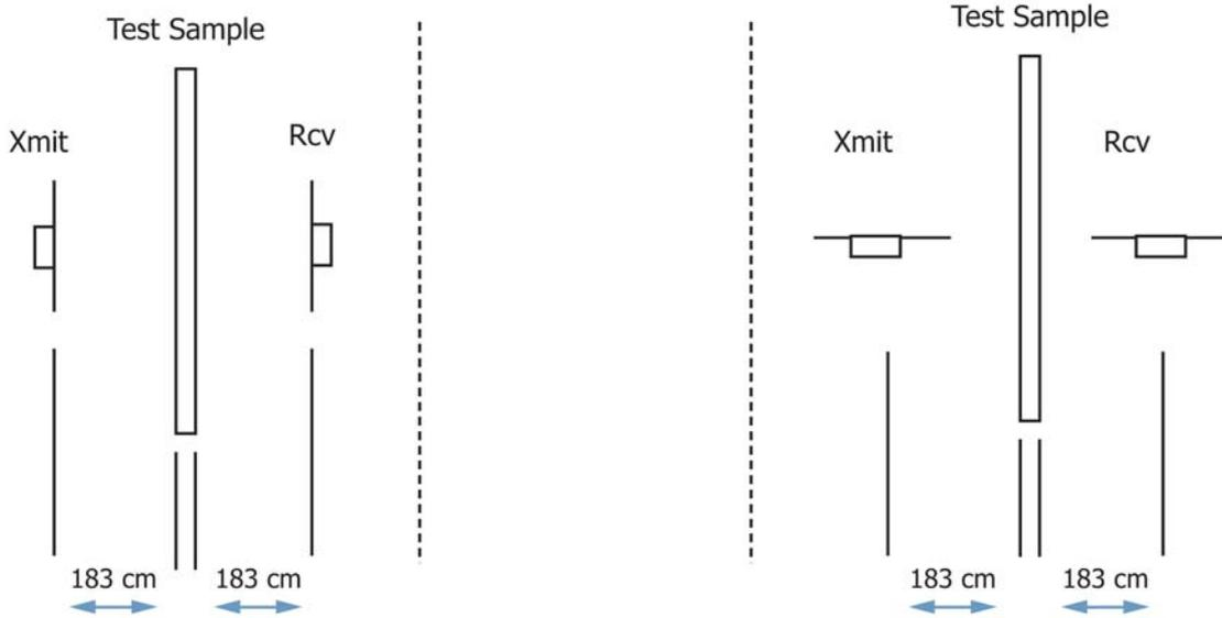
FIG. 2 Electric Field Antenna Positions (Dipoles and Monopoles)
